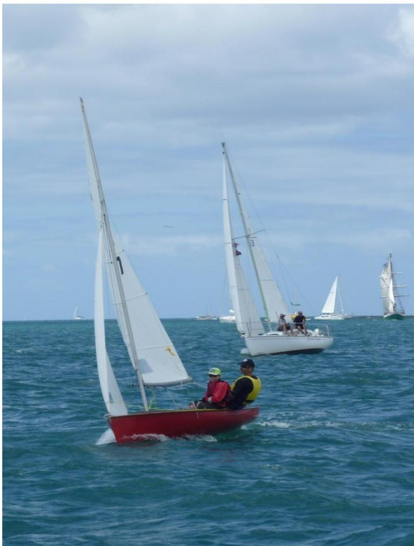
Check out what is meant by the jib and mainsail 'slot', and also the very baggy main that the Mistral has.
